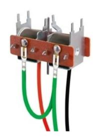
For 4 pin solenoids like the Peco shown One side the wires (shown in Green) are joined together these are connected to the centre solenoid output pin.
