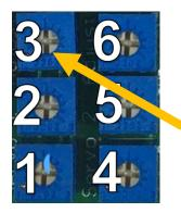
Step 7 -- Set the signal Clear upper position Turn the switch connected to input3 on, the Green LED next to input 3 will now be on, The Red LED must be off (Switch at input 1).
