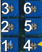
Step 9 -- Set the signal STOP Lower position Turn the switch connected to input 4 on, the Red LED next to input 4 will now be on.
