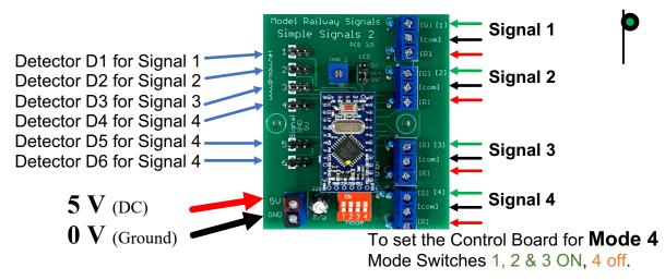
If you plan to use all four signals, please order 1 more train detector when you order. One **Mode 4** with 4 signals can be controlled by each **Signal 3.5** Control Board
