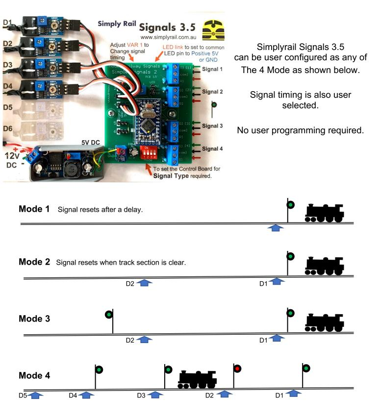
**Mode 1** is a simple way to start signalling your model railway. It is good for track where trains travel in only one direction.
