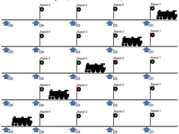
Signal 4 clears to green when the train has passed Detector 5
