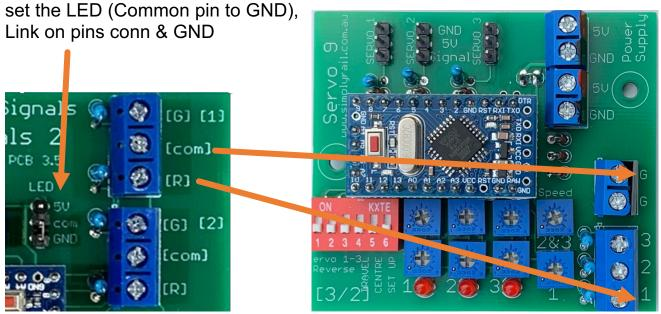
Connect the [com] ground pin to a ground input on the Simply Rail Servo controller.
