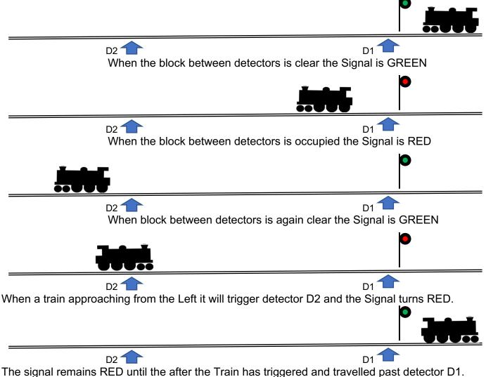
There is also a reset timer so the signal turns back to Green if only one detector was triggered.
