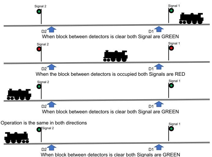
**Mode 3** effectively protects a block of track with trains traveling in either direction. This is an upgrade from **Mode 2** with signalling for both directions in visible areas.
