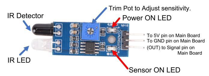
To set the Train Detector connect it to the main board.
