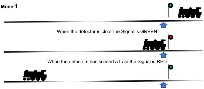
When the detector is clear and after a delay (10 to 60 Seconds) the Signal resets to GREEN
