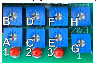
**Step 3** – To adjust the distance and direction of the travel for each servo.
