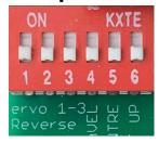
for Servo 1 turn Red <u>DIP 1 to ON</u>, for Servo 2 turn Red <u>DIP 2 to ON</u>. for Servo 3 turn Red <u>DIP 3 to ON</u>, Then readjust as per step 3
