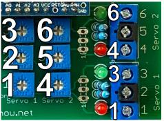
**Step 4** - To adjust the centre position of each servo. (Only for 3 position Signals)
