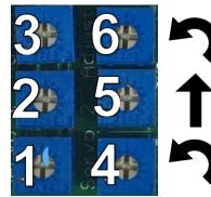
Step 1 - Before turning on the power, Please rotate each of the top and lower blue Trimpots anticlockwise, (1,3,4 & 6) Please rotate each of the middle blue Trimpots to the centre position, (2 & 5)
