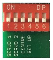
**Step 2** - To make it easy to position the servo, DP 3 will drive both servos to the middle of their travel and hold them in that position. Now turn on the power.
