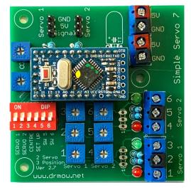
Once set-up, each servo is controlled by a simple switch. ON/OFF switch for two positions. ON/OFF/ON for three positions.
